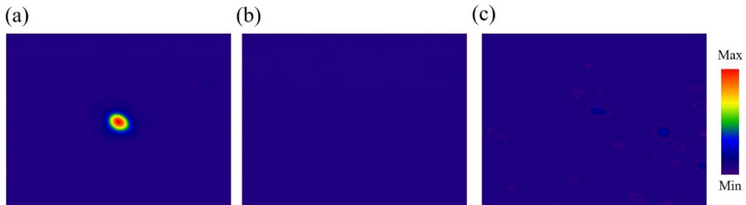
Figure S2. (a) The cross-section image of the focal spot in Figure 2(c) at X - Y plane. (b) The corresponding image after performing polarization analyzing at the orthogonal polarization state. (c) The recorded image with increased exposure time by twenty times.
